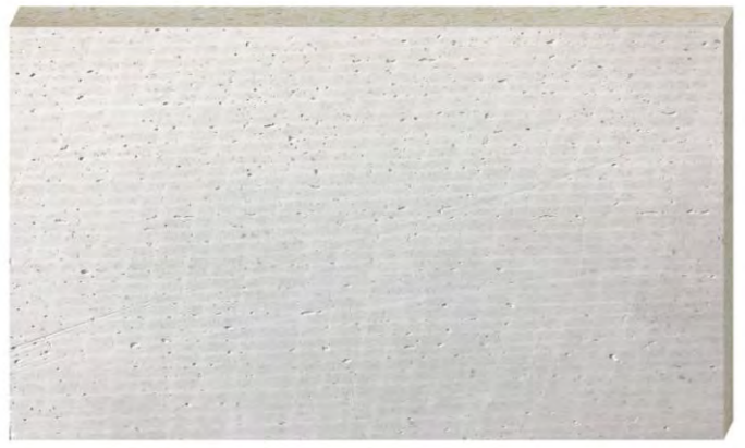
Standard MgO board surface with bubbles
