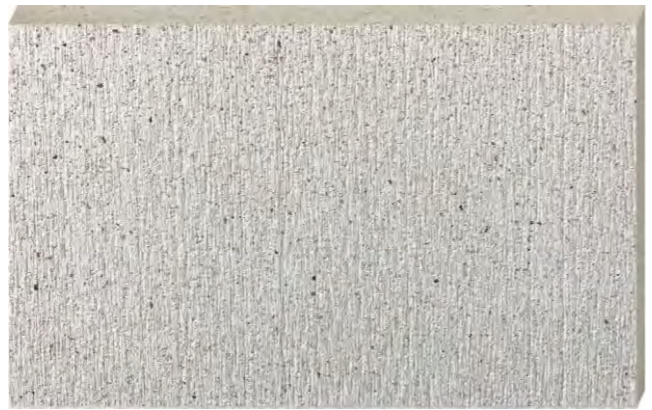
Sanded MgO board Using 100 purpose sanding paper sanding
